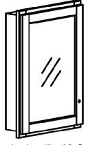
3D drawing shows Hinge left. For hinge right, replace the "L" in position 7 of the model number with a "R".
