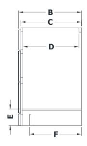
Cabinet height is 33 1/2". All dimensions are shown in inches rounded up or down to the nearest 1/8". Available in 16" and 18" deep, depth does not include doors and drawer fronts which add ¾".
