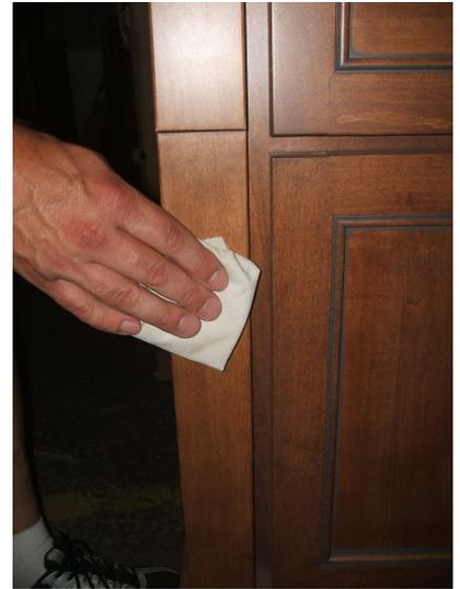
5. Inspect entire part for any defect, such as rub marks.
