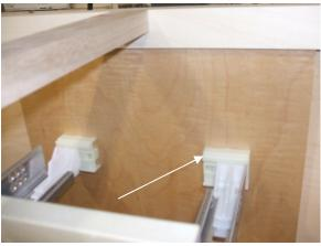
This shows the drawer plugs back in alignment after drawer was pulled out and properly re-aligned.
